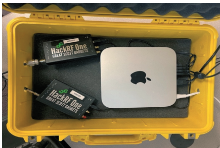
FIGURE 18: MAC MINI AND TWO HACKRF ONES IN A PELICAN CASE
