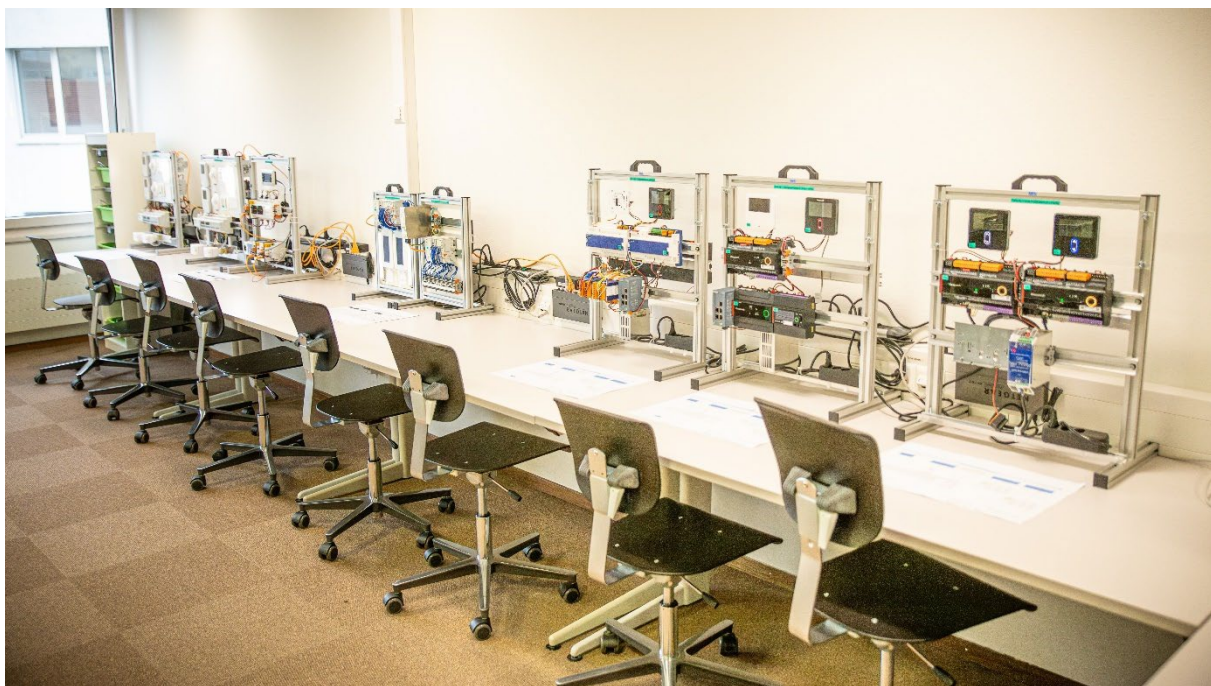
Figure 1. Cybersecurity test environment for building automation, installed at Lucerne University of Applied Sciences and Arts.
