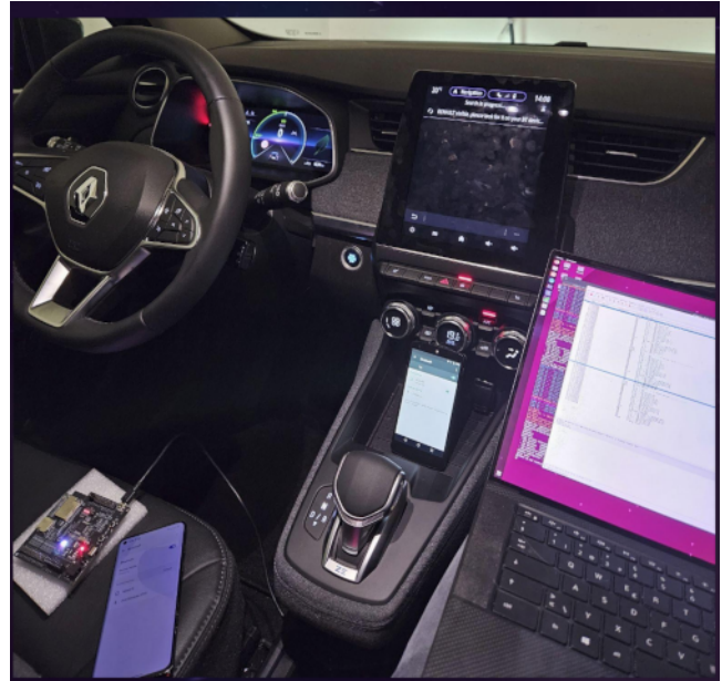
Figure 2: Testing a Renault Zoe (2021) with BlueToolkit.
