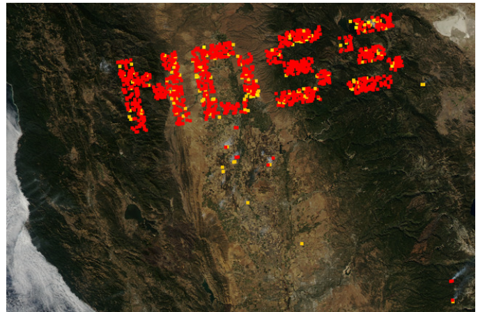
Fig. 1: An overshadowing signal from the attacker manipulates the infrared channels of satellite imagery to create fictitious fires in the resulting dataset.
