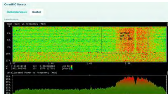
Demonstrator uses machine learning models to classify the electromagnetic spectrum in real time.
