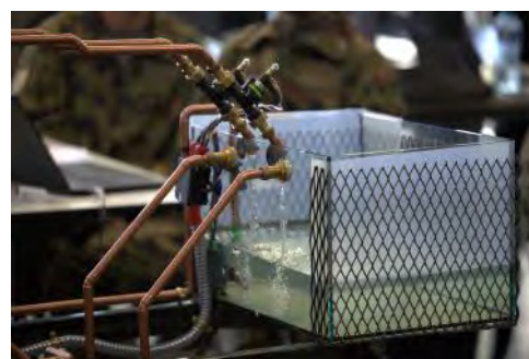
Model of a pumped storage power plant: CYD Campus ICS laboratory in Thun.
