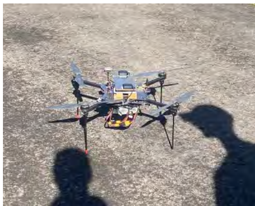
GPS jamming test on a drone.
