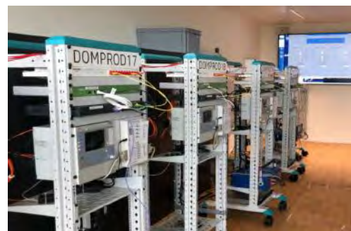
Krinflab: Reconstruction of a Swiss energy substation for the development of attack and defence strategies.
